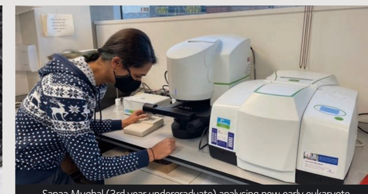
Sanaa Mughal (3rd year undergraduate) analysing new early eukaryote microfossils with Infrared spectroscopy to understand their organic composition.
