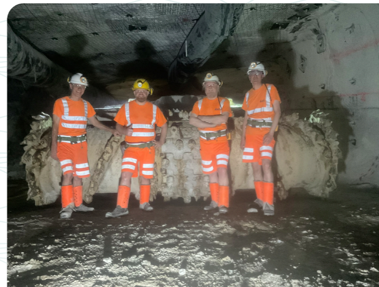
The visitors in front of the toothed rotating drum that extracts the polyhalite.
