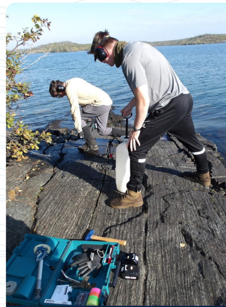
Sampling oriented cores in a pristine platform of banded iron formation. Water has to be pumped continuously through the drill to ensure the cores don't get hot during the sampling process.
